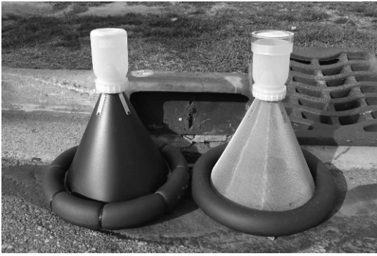
Fig. 1. Emergence traps next to a catch basin. The trap on the left is constructed of black plastic and the trap on the right is constructed of stainless steel mesh; all data presented in this study utilized the steel mesh trap style. The collection cup on the left is a closed inverted cup, while the cup on the right includes a removable lid with a screen mesh top.
