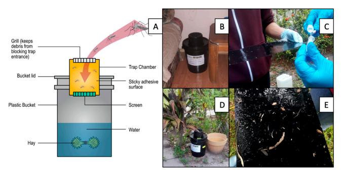
**Figure 2.** Pictorial diagram and field usage of the AGO trap (Source: CDC, Spring Star, King 5–modified). (**A**) Diagram of the features and components of the AGO trap. (**B**) Indoor placement of AGO. (**C**) Mosquito method of collection from glue board. (**D**) Outdoor placement of AGO. (**E**) Field view of a glue board that needs replacement.
