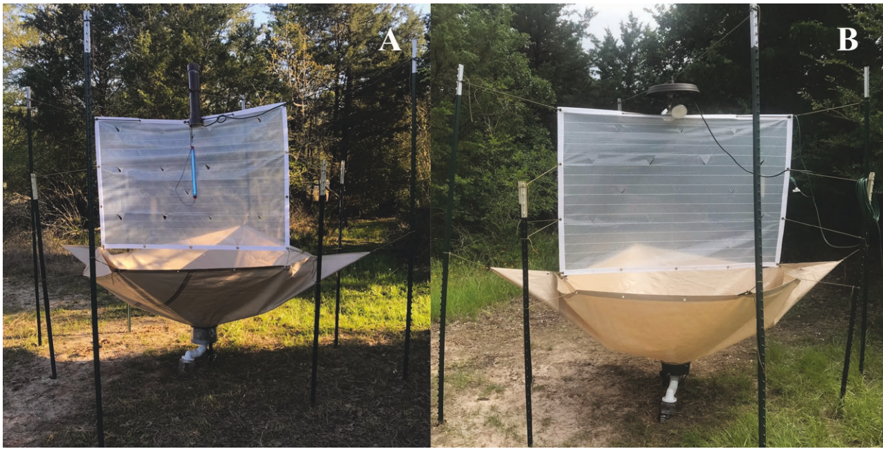
Fig. 2. Experimental vertical single panel traps with fluorescent blacklight A) and blue LED flood light B) tested in Texas, United States in 2019. Components include a transparent tarpaulin barrier panel, tarpaulin collecting funnel, lower aluminum funnel, white U-tube drainage tunnel, collection container and support T-posts with nylon ropes.
