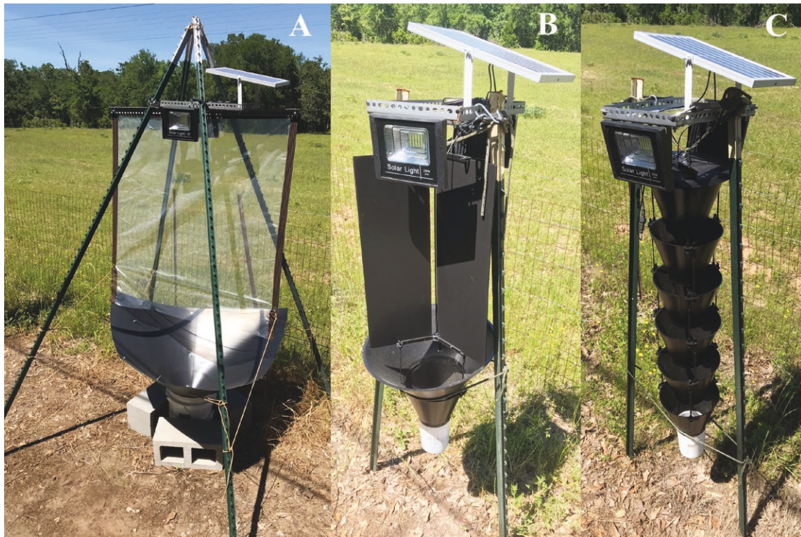
Fig. 3. Prototype traps deployed in Texas, United States comprising scaled-down vertical single panel trap A) tested in 2020, cross-vane trap B) tested in 2020, and multiple-funnel trap C) tested in 2020 and 2021. All traps have 2 identical large LED flood lights and solar panels with internal batteries mounted above.
